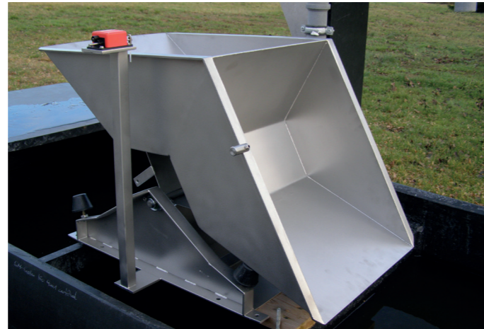
TIPPING COUNTERS - Tilt meter - for high time-resolved recording of seepage rates and flow rates made of PE or V2A steel. Tipping counter sizes 0.1 l and 20 l with data logger and adequate sampling.
