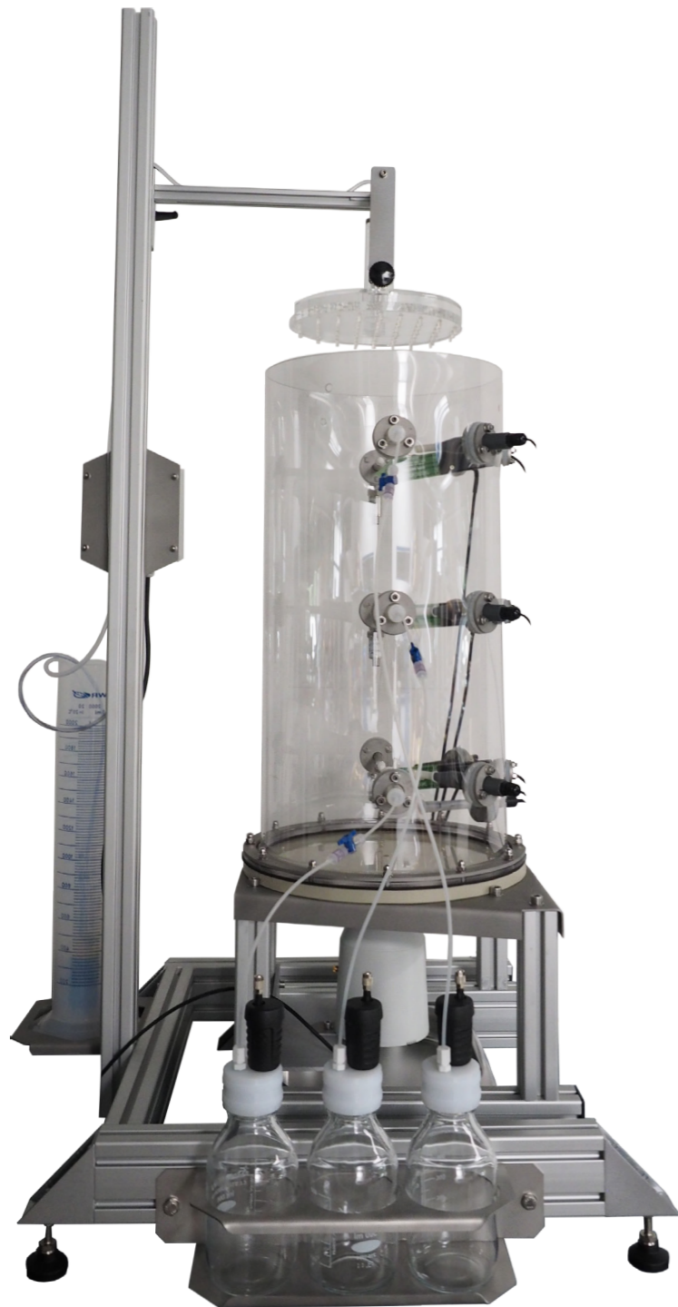
Laboratory lysimeter with PET lysimeter vessel
